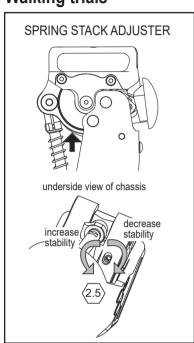
Fully extend limb to access the adjuster. Rotate the SPRING STACK ADJUSTER to achieve the required stability for the individual amputee. *Note: Audible clicks should be heard upon adjustment, and the adjuster is self locking.* Tighten the SPRING STACK to reduce stability. Release the SPRING STACK to increase stability - See above.
