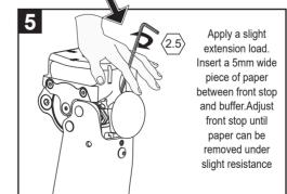
Any final adjustment required to alleviate rock should be by adjustment of the front stop.
